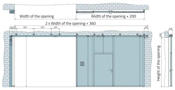
Installation is easy due to the low weight of the gate leaf, 20 kg/m2. It also reduces the requirements to the wall bearing capacity. The frameless design of the leaf eliminates the gate deformation at high temperatures and ensures the best protection against the spread of fire.
